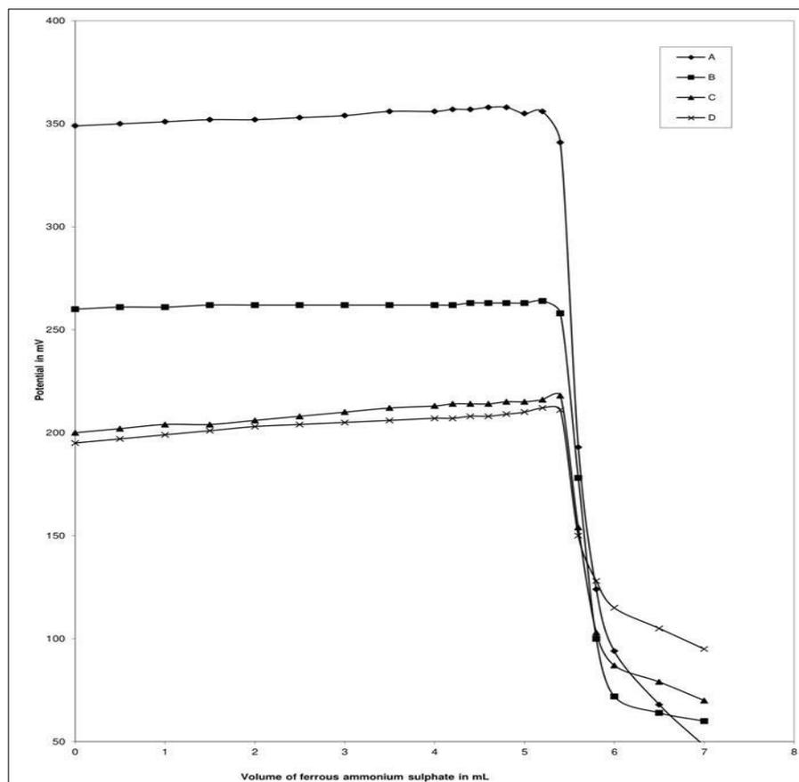
**Figure 8.** Effect of NTA concentration on the titration curves of 2.60 mg of vanadium (V) with  $9.30 \times 10^{-3}$  M iron (II) at pH 4.5 using platinum as an indicator electrode (Curve A 0.30 M; Curve B 0.20 M; Curve C 0.10 M; Curve D 0.01 M)
