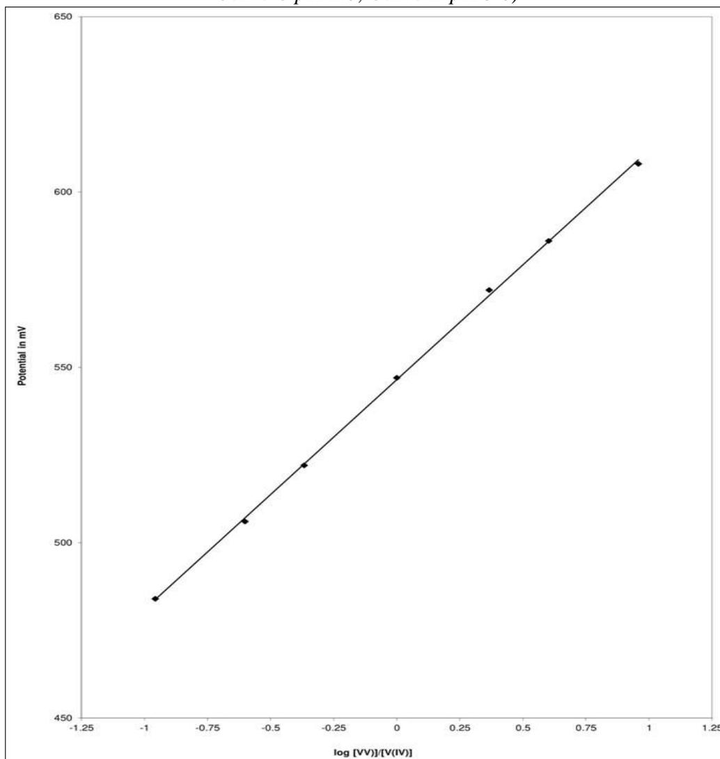
**Figure 2.** Sensitivity of graphite electrode towards V(V)-V(IV)-SCE
