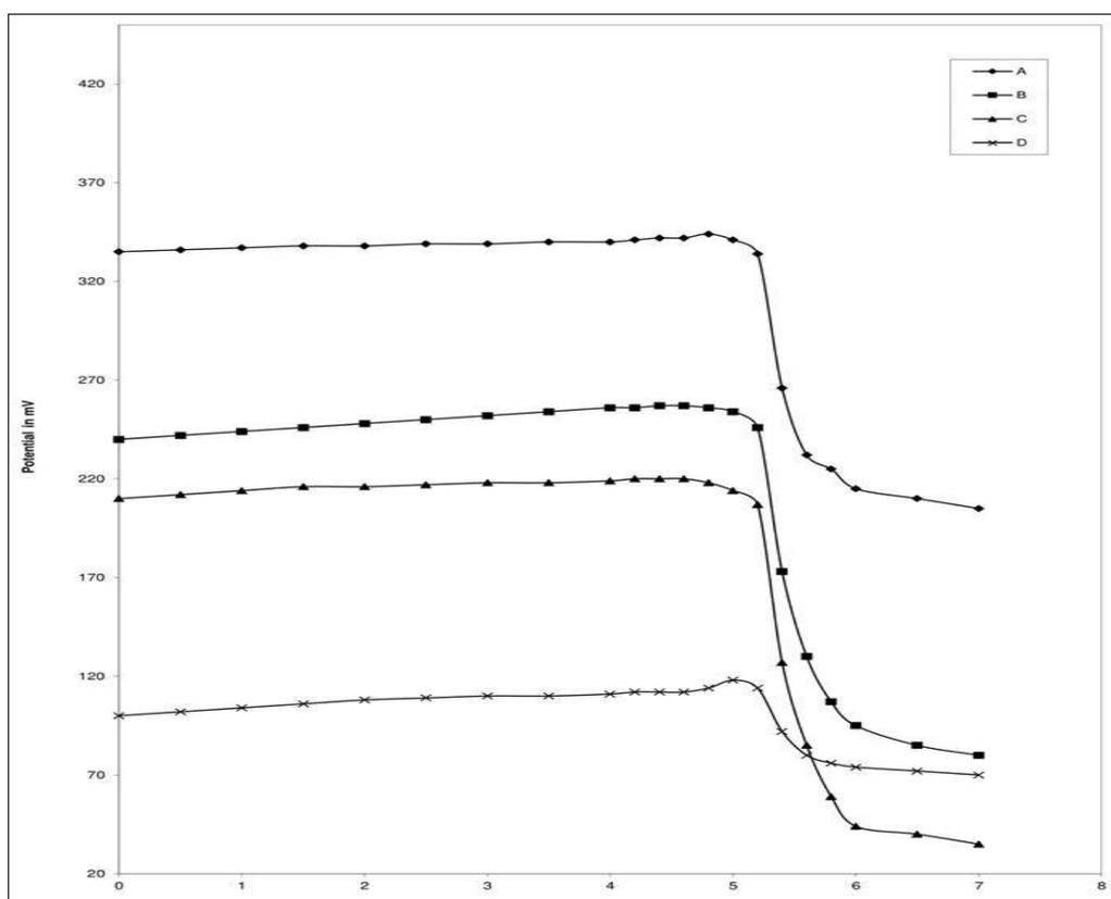
**Figure 6.** Potentiometric titration of 5.0 mL of  $1.02 \times 10^{-2}$  M vanadium (V) with  $9.3 \times 10^{-3}$  M iron (II) at various  $pH$  in the presence of 0.05 M NTA using platinum as an indicator electrode (Curve A  $pH$  3.0; Curve B  $pH$  4.0; Curve C  $pH$  5.0; Curve D  $pH$  6.0)
