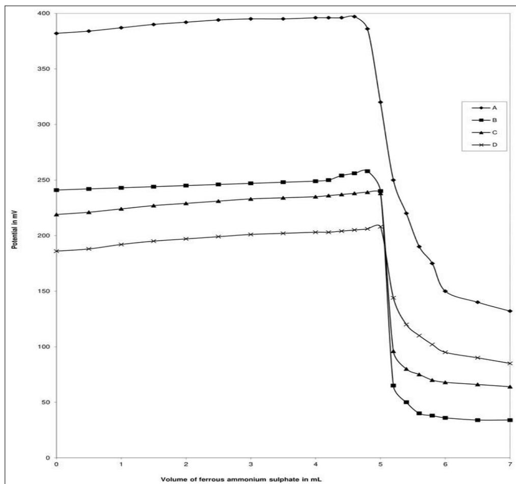
**Figure 7.** Potentiometric titration of 5.0 mL of  $1.06 \times 10^{-2}$  M vanadium (V) with  $9.64 \times 10^{-3}$  M iron (II) at various pH in the presence of 0.05 M DTPA using platinum as an indicator electrode (Curve A pH 3.5; Curve B pH 4.5; Curve C pH 5.5; Curve D pH 6.5)
