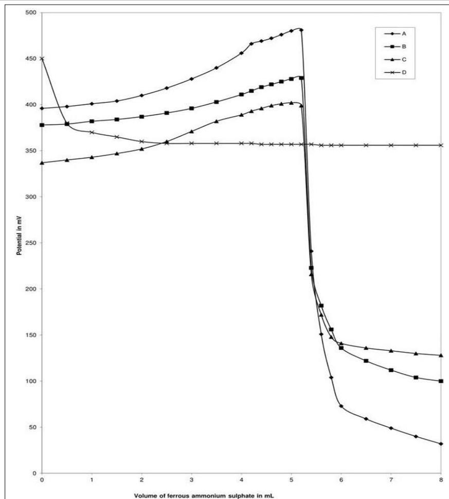
**Figure 9.** Effect of DTPA titration with 2.70 mg of vanadium (V) with  $9.64 \times 10^{-3}$  M iron (II) at pH 5.0 using platinum as an indicator electrode (Curve A 0.1 M; Curve B 0.05 M; Curve C 0.01 M; Curve D Absence of DTPA)
