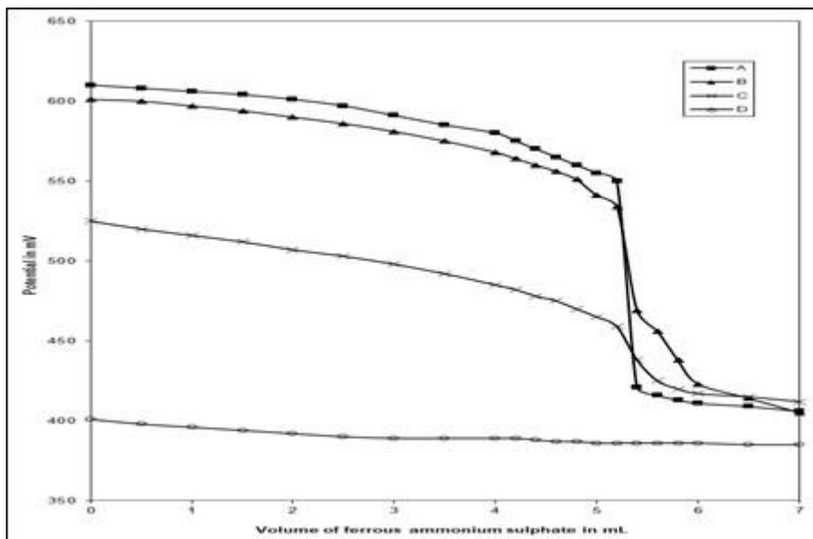
**Figure 1.** Potentiometric titration of 5.0 mL of  $1.05 \times 10^{-2}$  M vanadium (V) with  $9.9 \times 10^{-3}$  M iron (II) at various pH (Curve A pH 0.8; Curve B pH 1.0; Curve C pH 2.0; Curve D pH 3.0)
