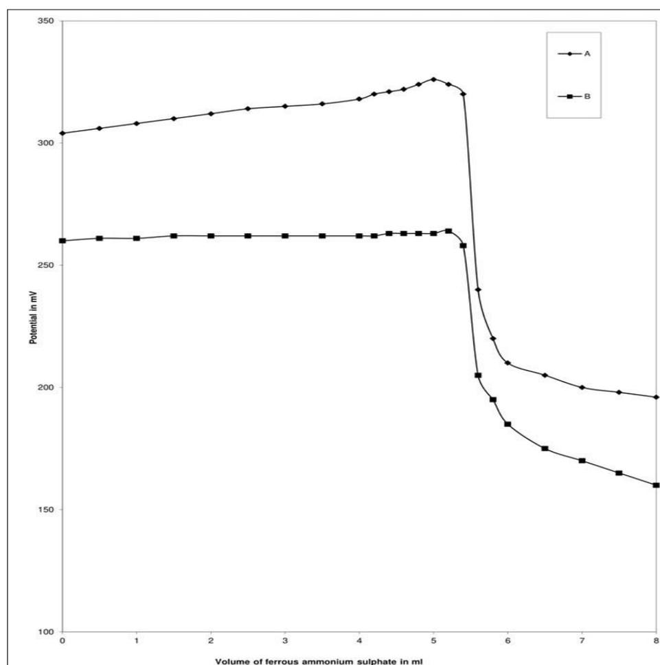
**Figure 10.** Potentiometric titration of 2.60 mg of vanadium (V) NTA using both platinum and graphite as indicator electrode Vs SCE (Curve A platinum; Curve B graphite)
