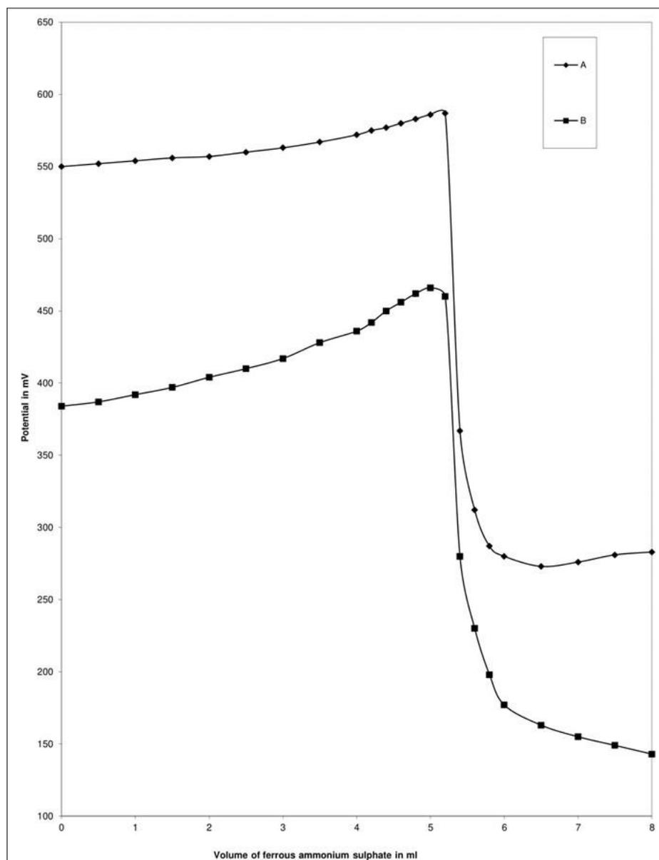
**Figure 11.** Potentiometric titration of 5.12 mg of vanadium (V) DTPA using both platinum and graphite as indicator electrode Vs SCE (Curve A platinum; Curve B graphite)
